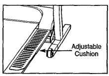
the cushions to level 2 or 1. It may be helpful to lift on the walking platform as you rotate the cushion. Note: The faster you run on the treadmill, or the heavier your weight, the firmer the cushioning system should be. Make sure that both cushions are at the same setting.
